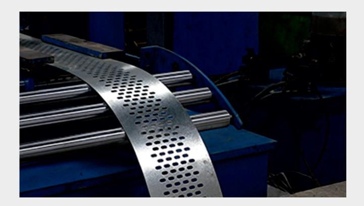
Aparna Rollform forming is a metal forming process that involves passing a strip of metal through a series of progressively shaped rolls, each of which shapes the metal a little more until the desired cross-sectional profile is achieved.
